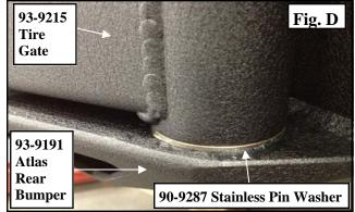
**Step 10:** Slide the main pin (90-9214) down through the hole in the Atlas rear bumper, stainless pin washer(s), tire gate, and into the lower bumper. Do not tighten at this time. (Fig E) *NOTE: The pin will be installed with the reduced shoulder on top.*
