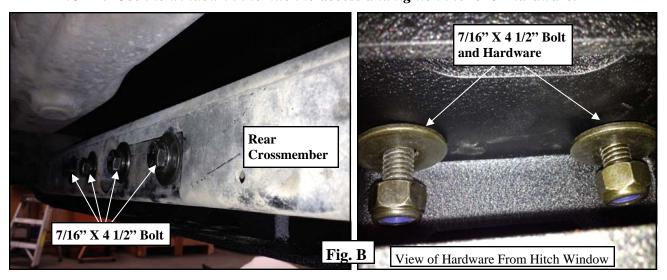
**Step 6:** Torque the **7/16**" bumper hardware to **55** ft./lbs. and **1/2**" hardware the **80** ft./lbs. (Fig B)
