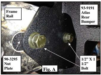
Step 4: Carefully raise the Atlas rear bumper (93-9191) against the outer frame rails. Secure to the outer frame rails and previously installed nut plates (90-3925) using the (4) supplied 1/2" X 1 1/2" bolts and washers. Leave the bolts loose at this time. (Fig A)
