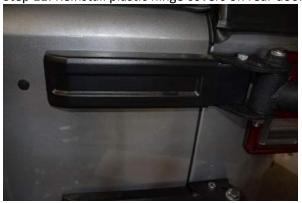
Step 12: With the help from a friend lift the new tire carrier into the hinges that you just installed on the body. Install the Allen headed bolt with adjusting nut on upper hinge and secure with nut. Install bolt on lower hinge and secure with nut. (note: only tighten finger tight at this point.)
