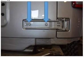
Step 3: Remove the 3 torx head bolts from the upper hinge on the body. Hinge should be free from Jeep.
