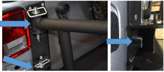
Step 21: Install the rubber bumper stops to the last two mounting holes with the provided hardware using the two button head bolts and secure with flange nuts. There are two sizes of stopper in the kit the longer one will go on top and the shorter one on bottom. (note: Do not over tighten or you will collapse the stopper.) The rear body mounting plate is now fully installed. Reinstall brake light housing and don't forget to plug the rear light harness back into the housing.
