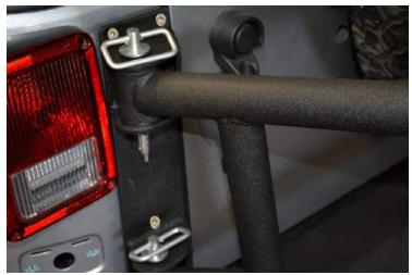
Step 20: Remove the quick release pins and pull the tire carrier to the open position. The body mounting bracket should be securely mounted to the body. Mark the last two mounting holes that were covered by the tire carrier when closed. Use center punch and hammer and lightly punch the center of your mark, drill pilot holes with 1/8" drill bit and then drill to final size with 1/4" drill bit.
