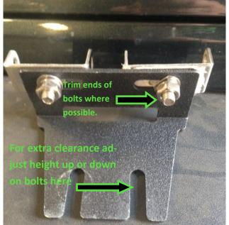
3) Place the mount in between the washers and the hinge itself as shown, tighten the bolts by inserting the wrench through the gap in the bracket. (Bracket should face towards the windshield)
