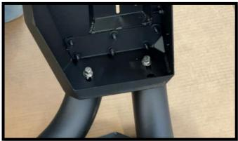
**STEP 6**: With assistance, install box assembly onto front and rear tubes as shown. Position the rear upper vinyl washer (item 14) and front upper vinyl washer (item 13) in between the tubes and base plate. Fasten down using 3/8" hex bolts (2), 3/8" flat washer (2) and 3/8" lock washer (2). Leave finger tight for later adjustment. Repeat steps for passenger side.
