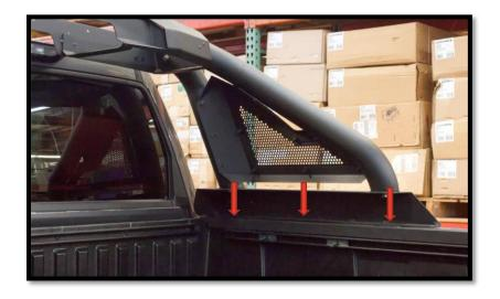
STEP 10: Mark any three holes along mounting bracket (per side) to attach sport bar, making sure the underside of the bed rail is free from any obstructions if possible. Some vehicles have perforations in the steel part of the bed rail. With caution, you may remove the plastic bed rail cover to verify where you are drilling is metal. Once this is determined, reinstall the plastic bed rail cover. Repeat steps for both sides. Remove Sport Bar once desired fit it achieved.
