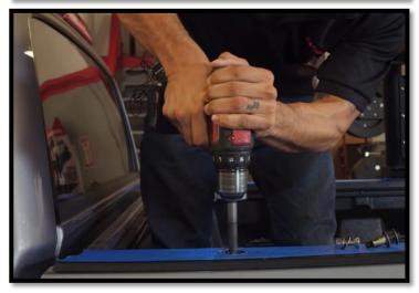
**STEP 13**: Use a 17/32" drill bit to make the hole where the rivet nuts will rest. It is important to use the correct size drill bit so that when the rivet nuts is installed and compressed, the knurl will catch onto the metal. Using any other size may result in the rivet nut spinning inside the hole. Apply automotive primer to any exposed metal.
