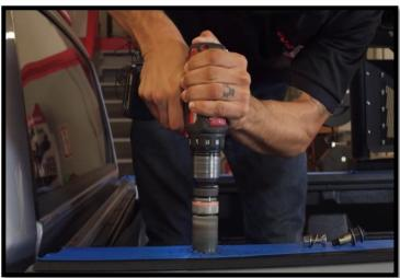
**STEP 12**: Use a hole saw (1 3/8" or smaller) to cut the plastic bed cover. Do not cut into the metal of the bed rail. If you do not have a hole saw, use a box cutter to make a 1"x1' square hole around the pilot hole.
