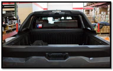
**STEP 17**: Place the sport bar over drilled mounting holes using the mounting base spacer as shown, both sides. If hole was drilled through top and bottom, attach the sport bar using (3)  $^3/_8$ " flat washers, (3)  $^3/_8$ " lock washers and (3)  $^3/_8$ " x 1  $^1/_4$ " flat head bolts, per side. If rivet nuts were installed, attach the sport bar using (3)  $^3/_8$ " x 1  $^1/_4$ " flat head bolts, per side. Make any final adjustments that may be needed.
