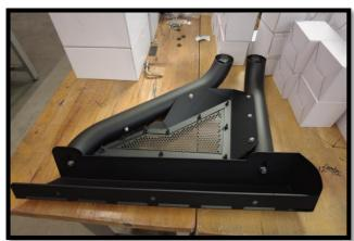
**STEP 5**: Install base plate onto front and rear tubes as shown. Position the rear bottom vinyl washer (item 16) and front bottom vinyl (item 15) in between the tubes and base plate. Fasten down using 3/8" hex bolts (2), 3/8" flat washer (2) and 3/8" lock washer (2). If you're planning on not using a tonneau cover with your Sport Bar, install the base plate cover on the bottom of the rear tube Reference images below. Leave hand tight for later adjustment. Repeat steps for passenger side.
