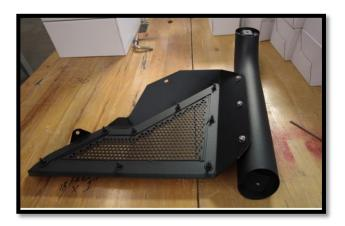
**STEP 3:** Attach front driver side tube (short) to the driver side mesh using ¼" button head screw (3), ¼" lock washer (3) and ¼" flat washer (3). Leave hand tight for later adjustment
