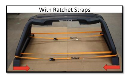
**STEP 9**: During adjustment, if the base plates overhang, you can use a clamp to secure it against the inside bed rail or use a pair of ratchet straps to keep it in place while adjusting it to your desired position.
