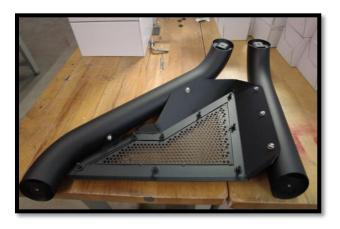
**STEP 4:** Attach rear driver side tube (long) to the driver side mesh using ¼" button head screw (2), ¼" lock washer (2) and ¼" flat washer (2). Leave hand tight for later adjustment. Repeat steps for passenger side.
