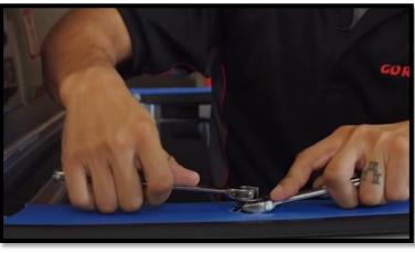
STEP 15: With the rivet nut positioned, use the provided rivet nut tool (item 25) to compress the rivet nut. Use a ¾" wrench to hold the spacer on the rivet nut tool and a 9/16" wrench to turn the head of the rivet nut tool. This will compress the rivet nut. Once tight, unscrew the bolt and repeat the steps for the remaining rivet nuts. OPTIONAL: You can use an impact gun on the head of the rivet nut tool or rivet nut gun to compress the rivet nut.
