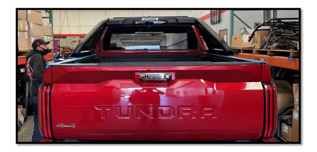
**STEP 8**: With assistance, position the Sport Bar 2.0 on the bed rails. Use painters tape to protect the OEM plastic. Begin to adjust the Sport Bar to your desired fit by moving the base plates, tubes and center box. Be sure that the vinyl spacers stay with the tubes to prevent metal to metal contact and preserve the life of the finish.
