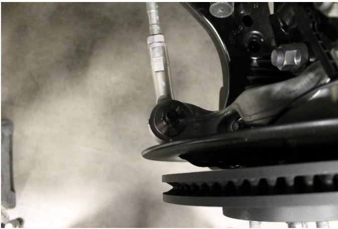
18. install / clip factory ABS wire harness onto strut, and install factory ABS Sensor onto knuckle
