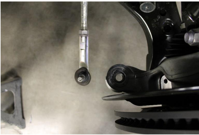
17. Install factory outer tie rod onto the knuckle
