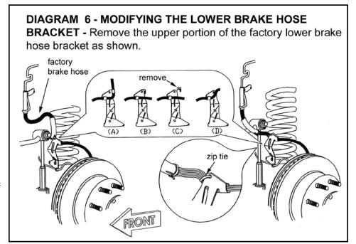
securing the stabilizer mount to the crossmember. It is not necessary to entirely remove the factory bracket.
