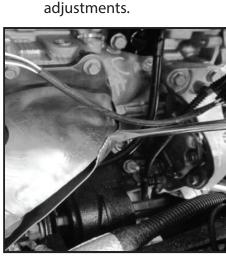
51 - With adjustments made insert tube and place mounting tab behind brake line mounting bracket. Secure 10mm bolt but do not tighten at this time. Final adjustment of air tube will be done later.
