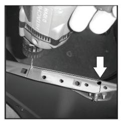
30 - Using a Dremmel tool or angle grinder fitted with a metal cutoff wheel cut fender along marked lines. Cut should start in the middle of outer cut line (arrow). Cut should be 1/8" away from rolled edge. Cut in each direction towards 7/32" terminating holes (arrows).
