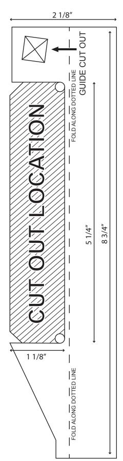
Cut out template using scissors or X-ATCO blade. The template is a (1:1) scale guide for cutting top of passenger side (LH) fender.
