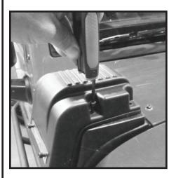
115 - With intake secure pull outer edge of "U" gasket away from intake until gasket rest flat against side of intake. 116 - Tighten all (6) caps head bolts.Do Not Over Tighten.A firm seal is all that is required.
