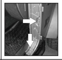
103 - Align lower fender holes with pinch weld mounting holes. Reuse bolts removed in step (15). Secure bolts but do not tighten at this time. 104 - Secure top of fender to inner fender frame.
