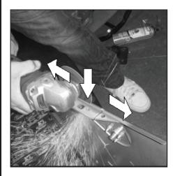
31 - Allow steel to cool before touching. Remove cut section from fender. Care should be taken when handling rough cut steel.
