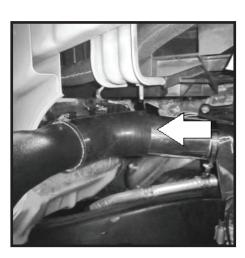
80 - Snorkel main body should rest in place as shown. Snorkel body should be fitted tight to inner frame. Some vehicles may require the pinch seam (arrow) to be rolled for proper fitment. Check antenna cable position.
