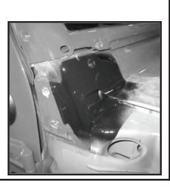
74 - Reinstall windshield bracket removed in step (2). Start and tighten the upper side M12 bolts and front M12 bolts as shown.
