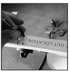
29- With guide holes marked and guide holes drawn drill 1/8" centering holes into fender. Use a 7/32" drill bit to enlarge 1/8" guide holes. NOTICE: A wood block should be placed under marked hole as described in steps 23&24. Wood block will protect the fender if drill bit grabs panel.
