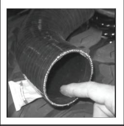
61 - Reinstall 90 deg elbow to lower air box. Align marks made in step (59). Slide 3" clamp onto elbow. With elbow placed against bottom face of lower air box tighten 3" clamp. Pull on elbow to insure it is secured tightly to inlet.
