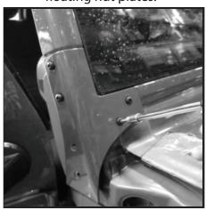
75 - If used, windshield light mounting brackets should be installed at this time.
