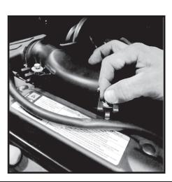
98- Adjust (4) air box sealing clamps full open. Clamps are designed to slip under lower air box flange and over flange and ribs of upper OE air box. Place clamps as shown (arrows). Secure but do not tighten clamps.
