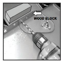
25- With spot welds cleared carefully remove upper cowl from fender.
