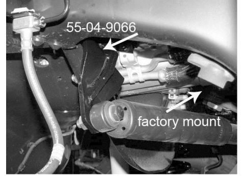
□ A bracket attaches the brake line / hose assembly to the outboard face of the frame rail, just forward of the coil spring tower. Unbolt this bracket from the frame.
