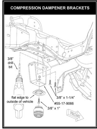
$\Box$  Attach the Superlift<sup>®</sup> bracket-to-frame using the supplied 3/8" x 1-1/2" bolts, pointing up, as shown. Place the washers on the frame side, install nyloc nuts and tighten (23).
