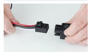
Red (+) is positive and black (-) is ground. These are the wires that connect to
