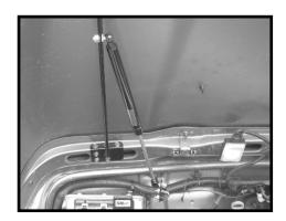
6. Make sure all hardware is tightened. Slowly lower hood while looking underneath to make sure no interference occurs. There may be a clearance issue in TJ/LJ models with the washer fluid reservoir. This can usually be fixed by grinding down the web between the cap and the hump in the reservoir.
