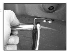
4. Bolt the lower ball stud mounting plate to the radiator brace rod about 6" from the fire wall using the supplied U-bolt. Orient the plate such that the unused hole is located above the rod. Insert a ball stud into the unused hole and tighten using a Nylock nut and washer. The ball should face outward as shown. Do this for both radiator brace rods.
