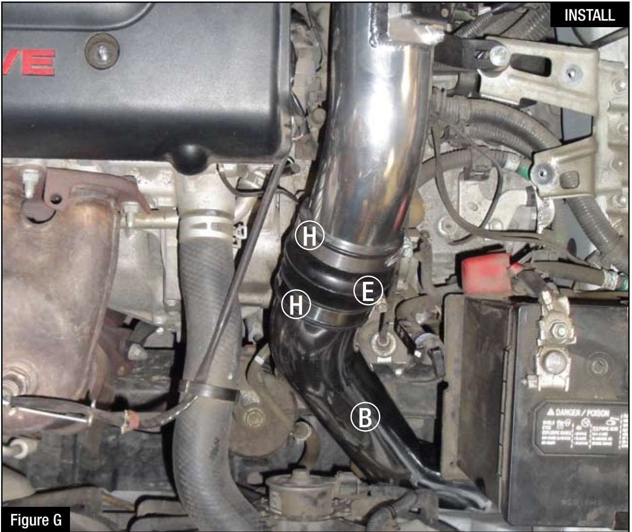
Figure G (For short ram install, skip to step 19) Step 13: Place 2 clamps (H) on hump coupler (E) and install the coupler onto the intake tube. Step 14: Install cold air tube (B) onto hump coupler.
