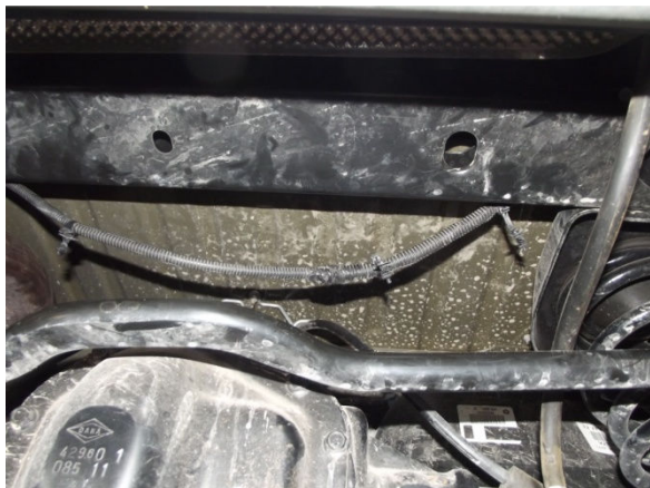
Photo 1 – Horizontal beam with wiring harness clips removed
