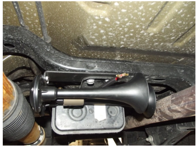
Photo 10 – Air horn bracket mounted under EVAP unit bracket
