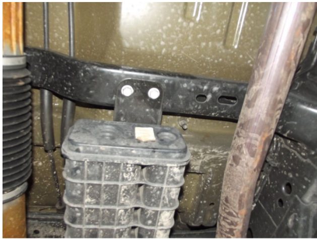
Photo 9 – EVAP canister. Note the two 5/8” mounting bolts
