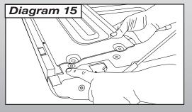
**D.** With the Tailgate Extrusion secured, carefully close the tailgate, being cautious not to strike the ends of the Tracks.
