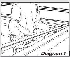
B. Unwrap the Tracks and locate the supplied Bed Clamps that are taped together along with the bolts and washers. Unwrap the Clamps and set them in the bed of the truck. Carefully place the Tracks on the bedrails (*Diagram 7*) and key them onto the Housing Stems (*Diagram 8*), being sure that the Handle is properly engaged into the Tracks.
