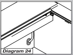
G. Always make sure the Pull-Strap is securely clipped to a fixed point in the bed.
