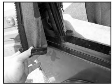
2. Unsnap the sides of the top and remove the top from the front tracking. Fold the front portion to the rear.
