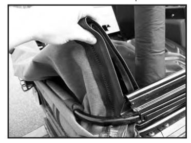
4. Open the boot and wrap it around the soft top and frame. Snap the boot closed around the top.
